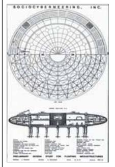
From the tops of these structures, a cylindrical concrete conduit extends 150 feet above the ocean surface. At surface level, it is encircled by a floating dock system, which rises and falls with the tides and accommodates both surface and submersible craft.
